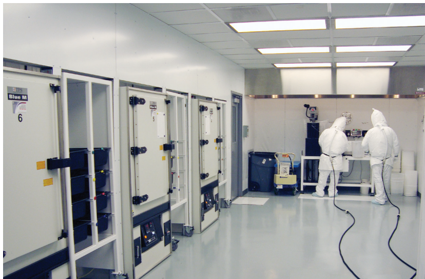
Urethane production in ISO Class 7 clean room
